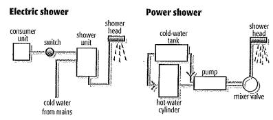
Unlike the electric shower, the power shower uses water which has already been heated in the central heating system. Firstly, hot water is taken from the hot water cylinder, while cold water arrives from the cold water tank. Then the hot and cold water is pumped into the shower by a special pump. Finally, the water is mixed by a valve before it comes out of the shower head.
